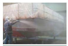
SPRAY APPLICATION to 3mm coating thickness of Eraspray ESM900 grey via high pressure impingement mixing equipment.
