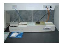
Coefficient of Friction Tester
