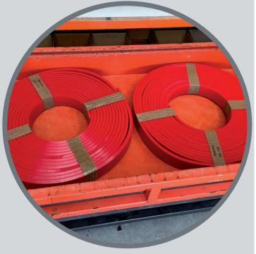
Coiled PU conveyor skirting (18M lengths) ready for transport.
